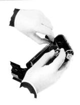
the holder into the round hole of the spool. This brings the slotted end of the spool next to the winding key. The Kodak is now ready for reloading.
