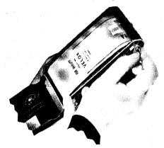
Turn the winding key once or twice to bind the paper on the reel, and be sure that the paper is started straight. Close the back, pressing it so that the spring lock snaps into place, securely fastening the back.
