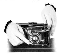
All being ready, press the exposure lever carefully, once to open, time the exposure by a watch, and again press the exposure lever to close the shutter.
