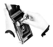
Remove the empty spool and place it in the spool holder in the winding end of the camera, fitting the pin on
