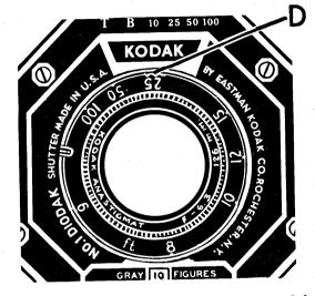
The distance between the subject and Kodak can be estimated without measuring, when the subject is beyond fifteen feet; for instance, if the focus is set at 25 feet (the usual distance for ordinary street scenes) the sharpest part of the picture will be the objects at that distance from the camera, but everything from about 18 to about 45 feet will be in good focus.
