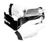
loosening. Draw out the key and remove the film. Fold under about half-
