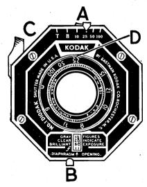
A—Speed Indicator B—Stop Opening Lever D—Focus Pointer
