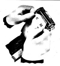
Remove the paper band and pass the protective paper over the two rollers. Thread the paper through the longer slit in the empty reel, as far as it will go.
